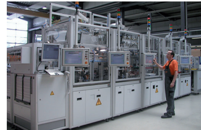
Assembly system for car injection components with integrated laser-welding and laser-marking (data matrix code)
